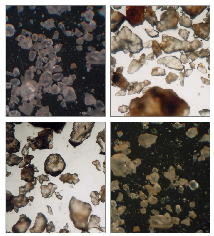
The limescale crystals depicted here have been transformed into aragonite in the UMH water purification process. Thanks to the rounded shape of the crystals, there is no tendency for scale to adhere to surfaces. The sand-like residues are flushed out and existing limescale is gradually broken down.
