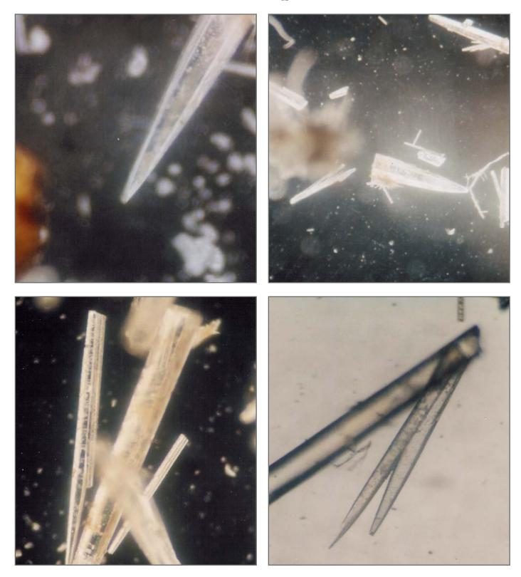
These sharp calcite crystals are formed when normal tap water is heated, and tend to result in massive limescale deposits.
